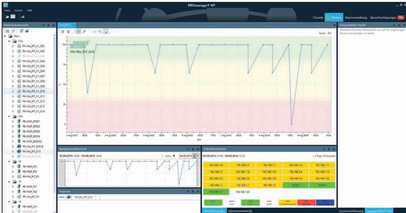
PROmanage NT provides the operator with all important information at a glance: for example, the overall network status over time with a graphic emphasis based on the principle of stop light colours (top centre), a device matrix with colour evaluation of the current status (bottom right) and the overview of all monitored networks with quick control access (left side panel).
